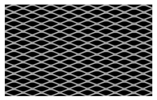
LW Pitch:19.05mmStrand Width:1.70mmSW Pitch:7.43mmThickness:0.90mmWeight:1.12 kg / m2Open Area:54%
